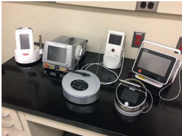
Figure 1.28 Various diode lasers for oral applications (from left to right): Sirona blue light; KaVo 980 nm; Spectralaser (980 nm); Ivoclar 810 nm; Epic (940 nm, Biolase); and the Alta Diode (975 nm) laser with automatic power control (APC) (Biolase). Source: Dr. Georgios E. Romanos.
