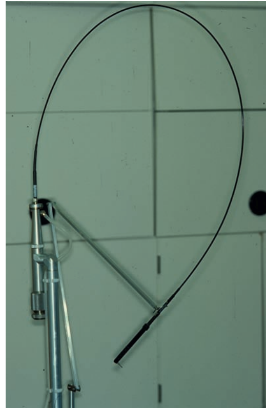
Figure 1.9 Hollow guide of a CO 2 laser presenting the flexible delivery system for oral applications. Source: Dr. Georgios E Romanos.
