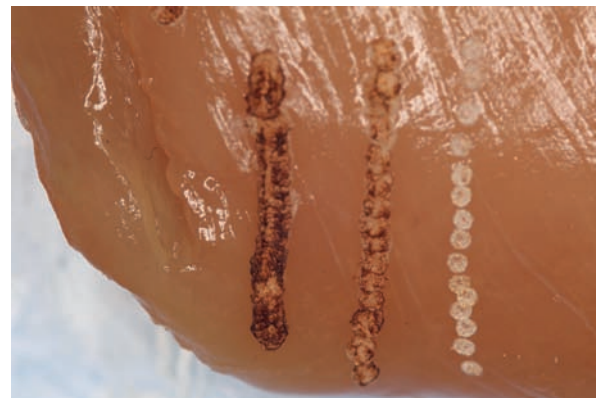
Figure 1.43 Photothermal effects of a 3W-CO 2 laser on soft tissues (chicken breast) using a continuous wave (left), pulsed mode (middle), and superpulsed mode (right). The thermal effects demonstrate changes in the tissue. Source: Dr. Georgios E Romanos
