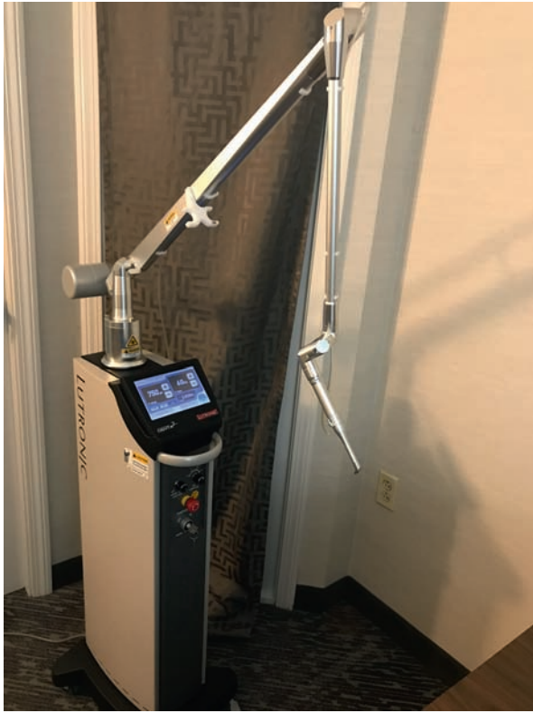
Figure 1.8 Articulated arm for a CO 2 laser application in the modern CO 2 laser (Denta 2, Lutronic, GPT dental, Fairfield, NE, USA).
